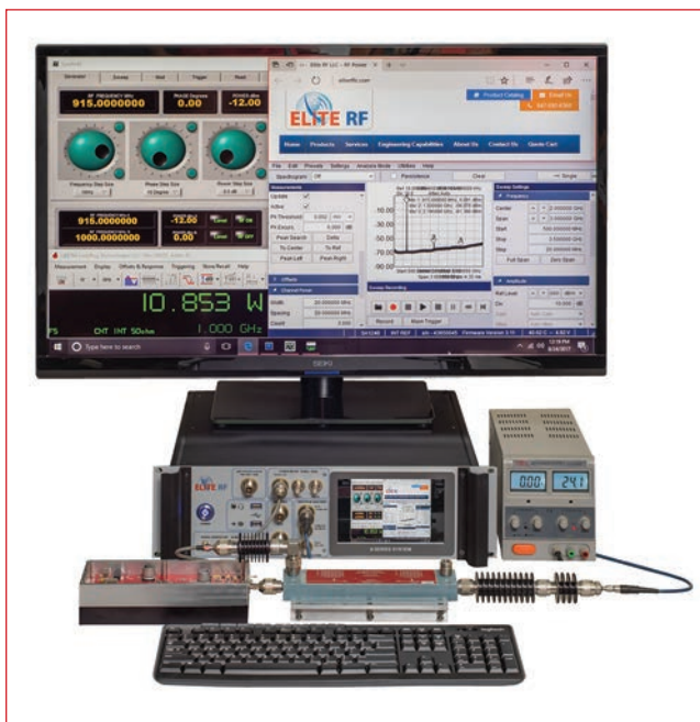
▲ Fig. 1 Testing a 900 MHz, 65 W power amplifier.
