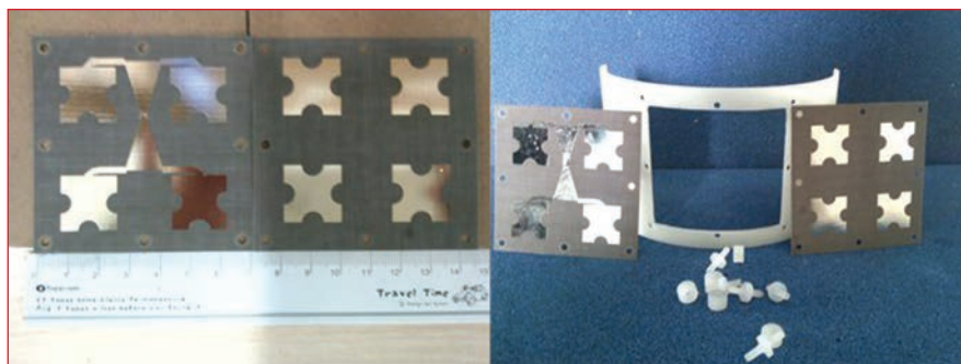
▲ Fig. 5 Prototype conformal antenna.
